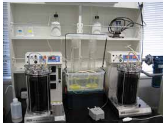
Lab equipment for producing biogas through anaerobic degradation of halophytic plants (Photo by Natalya Akinshina)
