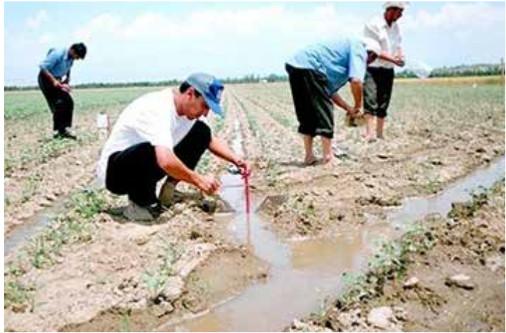
Water discharge measurement: demonstration and dissemination of technologies for more efficient use of irrigation water, WPI-PL project in Fergana Valley. Photo by IWMI.
