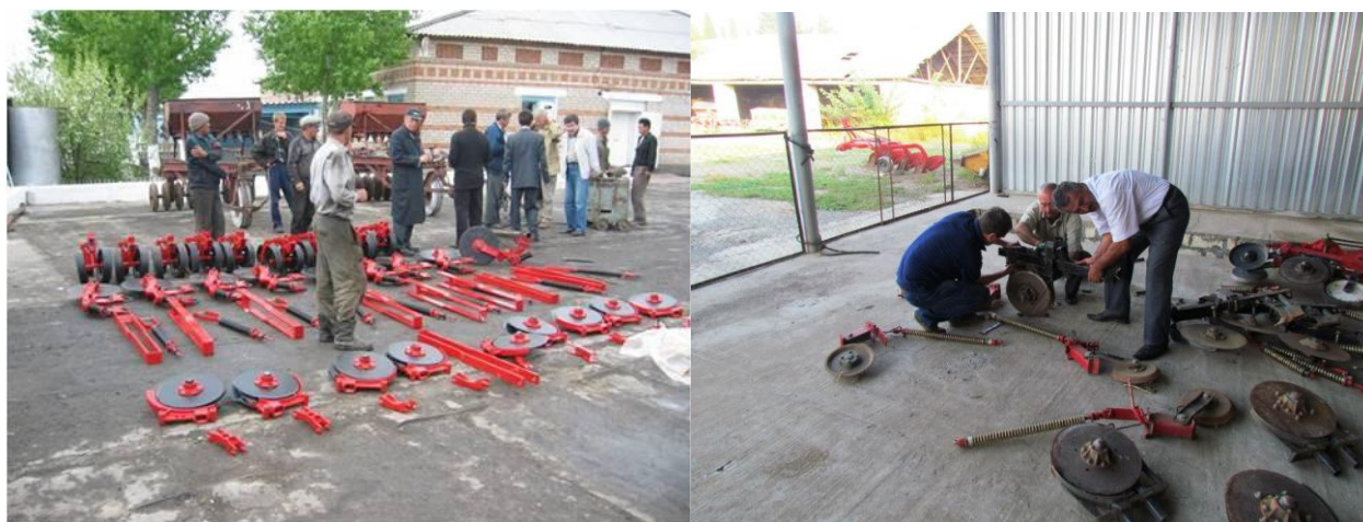
A B Figure 6. Assembling no-till drill in Kazakhstan (A) and Azerbaijan (B)
