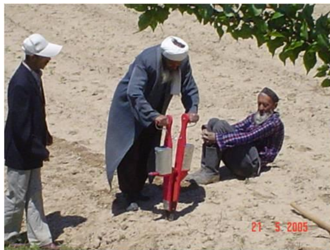
Figure 8. Adoption and promotion of CA requires proper tools such as jab planter
