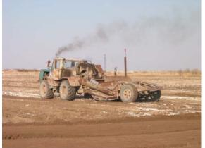
Photo 8. A receiver is mounted on the leveling equipment.
