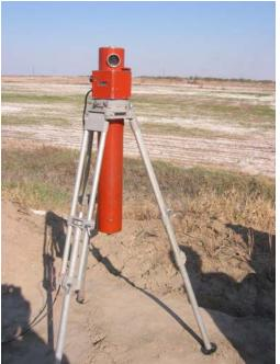
Photo 7. A rotating laser light source.
