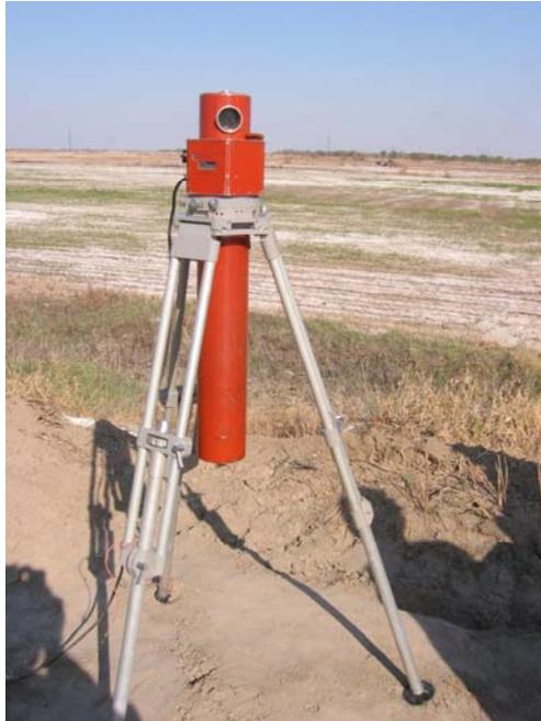
**Photo 7. A rotating laser light source.**
