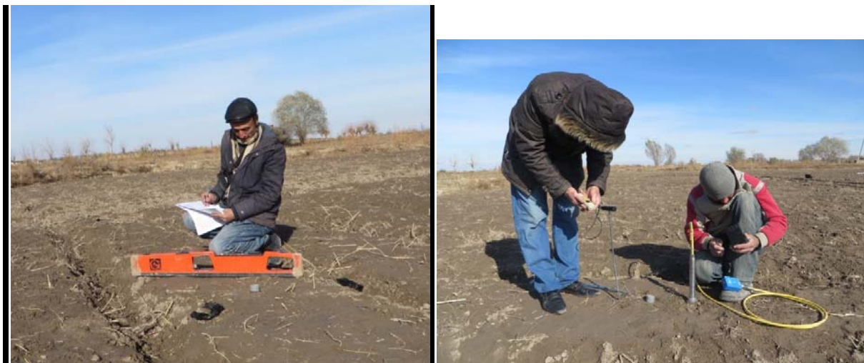
Appendix 4 Soil salinity ( \text{dS m}^{-1} ) measured by EM38 instrument in Chimbay site, 2015
